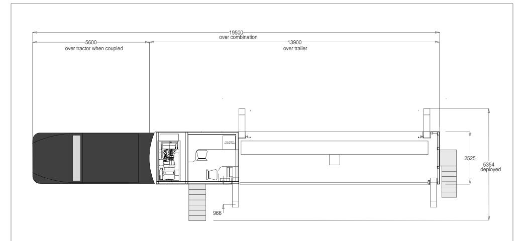
Footprint Plan View of Big TV Screen trailer with screen only deployed
